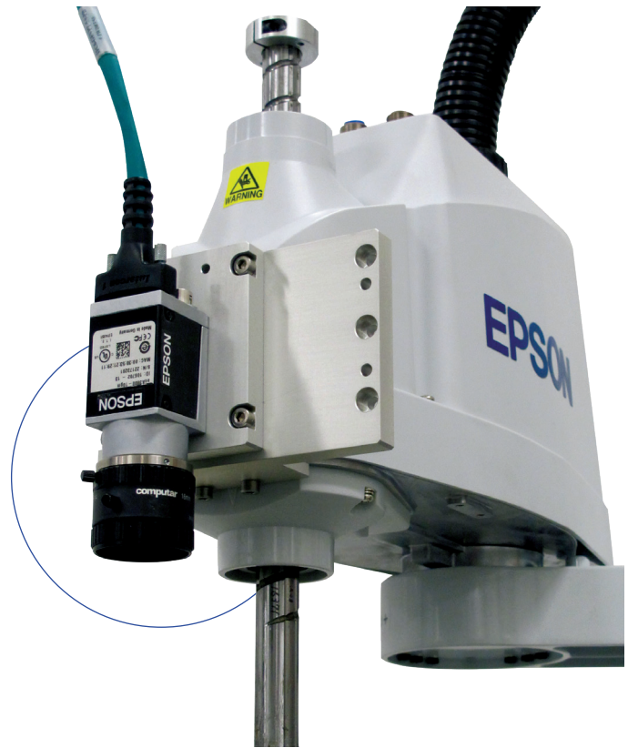
T-Series robot shown with mobile-mounted camera as part of the Epson Vision Guide option.
